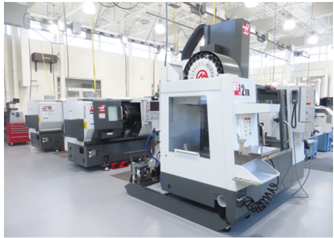
The 10,000 square foot QVCC Advanced Manufacturing Technology Center featuring a 5-axis Haas VF-2TR, along with two Haas ST-20 turning centers. Capable of simultaneous five-axis machining, the VF-2TR represents the highest level of technology within the center.
