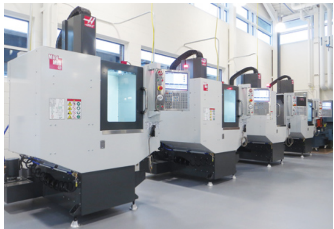
Rounding out the CNC machines in place within QVCC's all-new Advanced Manufacturing Technology Center are four Haas Mini Mill vertical machining centers
